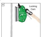
3. Place the Cable Sleeve onto the vertical cable so the cable is seated in the cable slot and release the locking lever and locking cam lever to complete attachment to the vertical cable (Figure 5).
